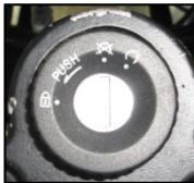
“○” mark... The key is turned to the “○” mark position, the power is turned on, the engine can be started, and the key cannot be taken out;
